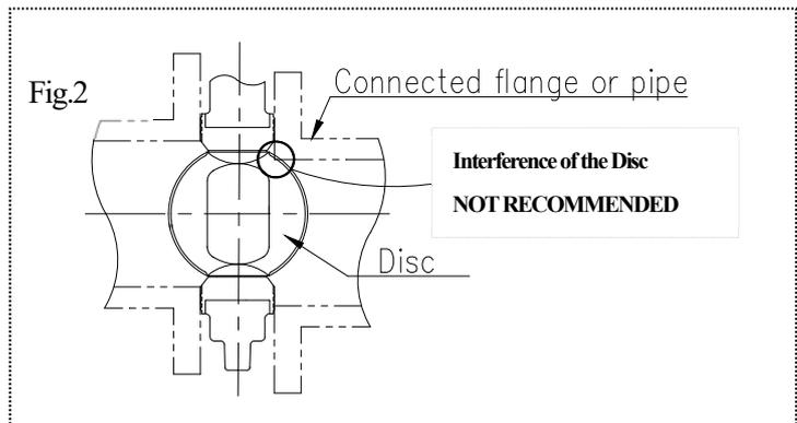
In case of the thick of the connection part (flange and pipe) is too thick shave the flange or the pipe inside order to avoid the contact of pipe and disk. If inside diameter of the connection part is larger than size D, shaving is not necessity.
