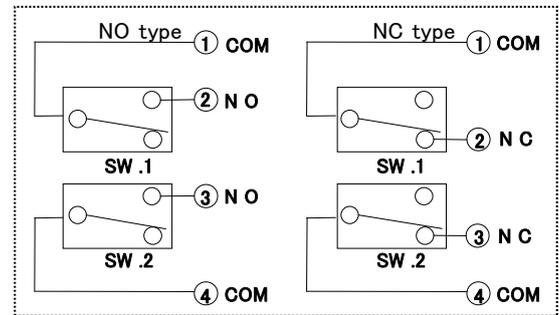
SW.1: Contact closes when valve is closed (double acting/air to open)
