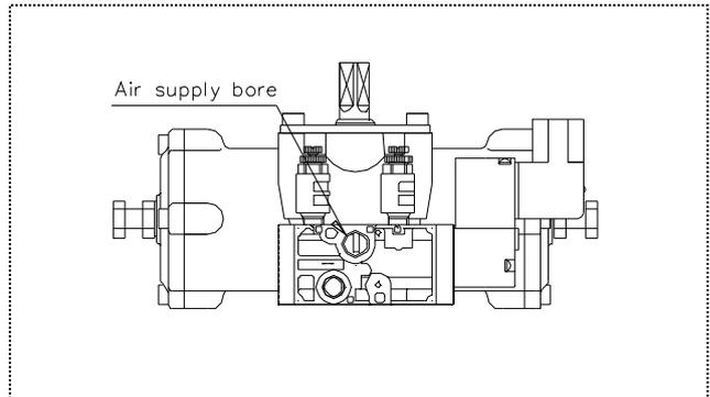
(Fig.2) Solenoid valve, Pressure reducing valve with filter
