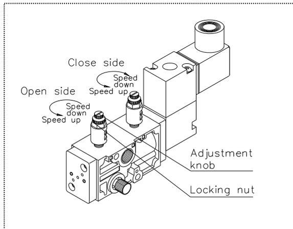
For Double action type with speed controller
