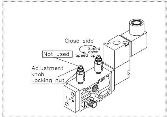
For Single action type with speed controller
