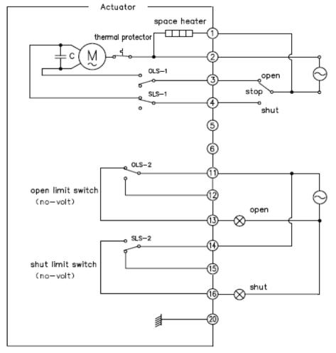
NOTE :The wiring diagram shows when the right full-open operation ends.
