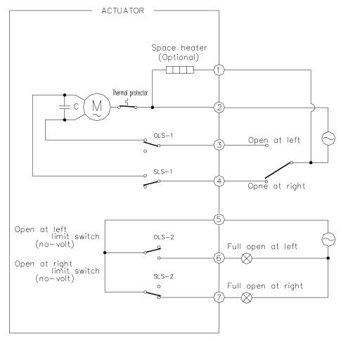
NOTE :The wiring diagram shows when the right full-open operation ends.
