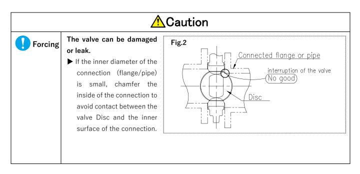
The butterfly valve is designed to be used for piping of various materials. However, especially when a large wall thickness of the connecting part (flange pipe) with the valve is used, it is necessary to chamfer the inner end of the connecting part in order to avoid contact between the valve Disc and the inner surface of the connecting part. There is no problem if the inner diameter of the connecting part is equal to or greater than the following value.
