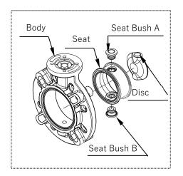
**5)** Put the disc [2] of the seat disc set in half-open position, align the stem hole of the body [1] with the stem hole of the seat disc set and fit the seat [3] inside the body [1].
