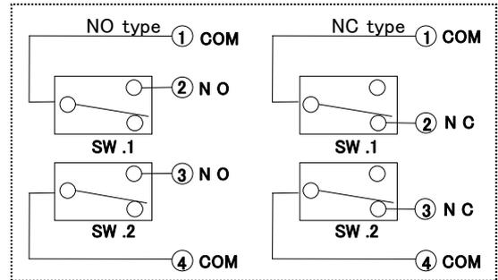
SW.1: Contact closes when valve is closed (double acting/air to open)
