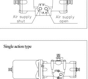
Air to open type: Air supply open Air to close type: Air supply shut
