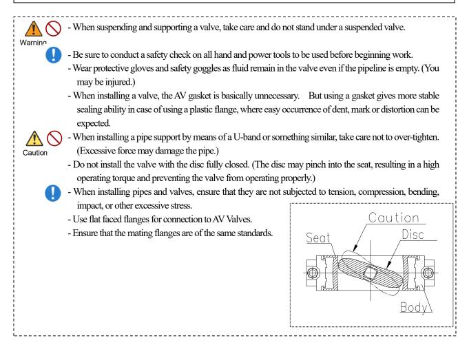
Care must be used during piping installation to ensure that the pipes or flanges are properly aligned so that the valve disc does not contact them in any setting. Misalignment as in Figure below will result in damage
