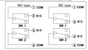
SW.1: Contact closes when valve is closed (double acting/air to open) Contact closes when valve is opened (air to shut)
