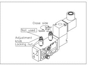
For Single action type with speed controller
