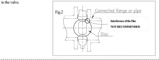
In case of the thick of the connection part (flange and pipe) is too thick shave the flange or the pipe inside order to avoid the contact of pipe and disk. If inside diameter of the connection part is larger than size D, shaving is not necessity.
